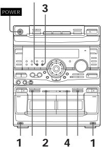
Press § EJECT and insert a recorded tape in deck A and a blank tape in deck B.
